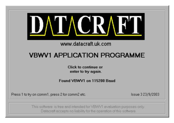
The software looks for a VBWV1 board connected to Comm1, if one is found left click to go to the next screen. To try again press enter or 1,2,3 or 4 to try different comm ports.
